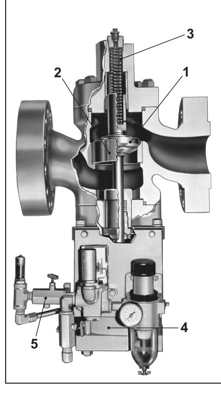
A stem-guided, stainless steel, poppet-type disc (Item 1) closes against the stainless steel seat (Item 2). Closing force is normally supplied by accumulator pressure acting on the valve disc; at very low accumulator pressure, such as is experienced when starting up, a stainless steel spring (Item 3) supplies sufficient pressure on the disc to ensure closure.
