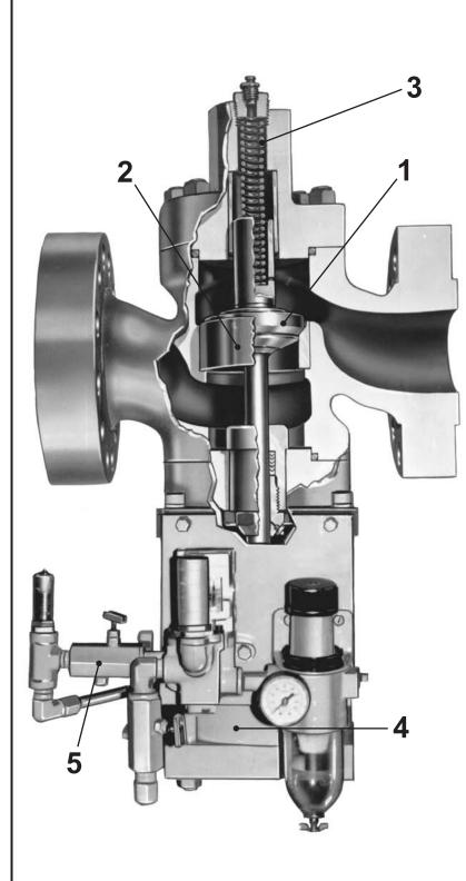
A stem-guided, stainless steel, poppet-type disc (Item 1) closes against the stainless steel seat (Item 2). Closing force is normally supplied by accumulator pressure acting on the valve disc; at very low accumulator pressure, such as is experienced when starting up, a stainless steel spring (Item 3) supplies sufficient pressure on the disc to ensure closure.
